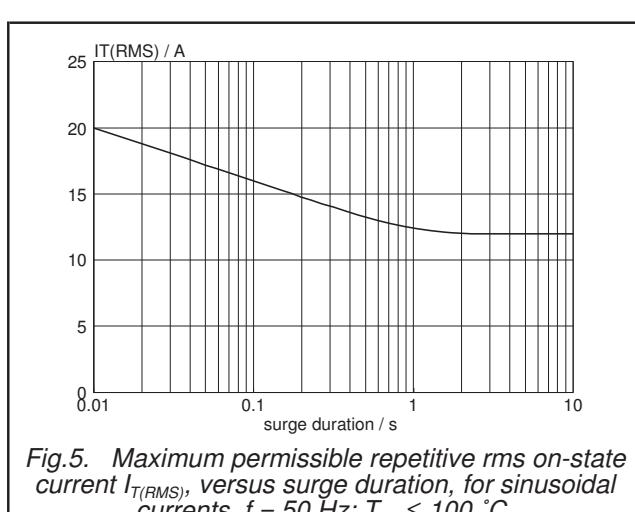
Fig.5. Maximum permissible repetitive rms on-state current  $I_{T(RMS)}$ , versus surge duration, for sinusoidal currents,  $f = 50$  Hz;  $T_{mb} \leq 100^\circ\text{C}$ .
