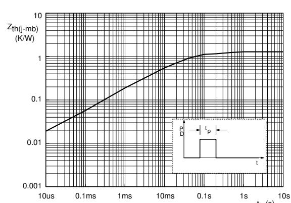
Fig.11. Transient thermal impedance  $Z_{th(j\text{-mb})}$ , versus pulse width  $t_p$ .
