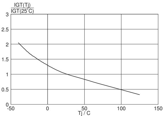
Fig.7. Normalised gate trigger current
