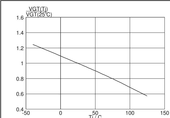
Fig.7. Normalised gate trigger voltage  $V_{GT}(T_j)/V_{GT}(25^\circ\text{C})$ , versus junction temperature  $T_j$ .
