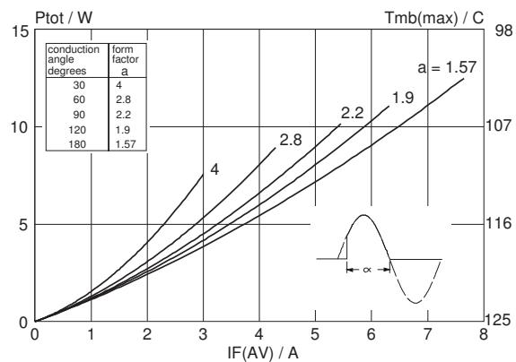
Fig.2. Maximum on-state dissipation,  $P_{tot}$ , versus average on-state current,  $IT_{(AV)}$ , where  $a = \text{form factor} = I_{T(RMS)}/I_{T(AV)}$ .
