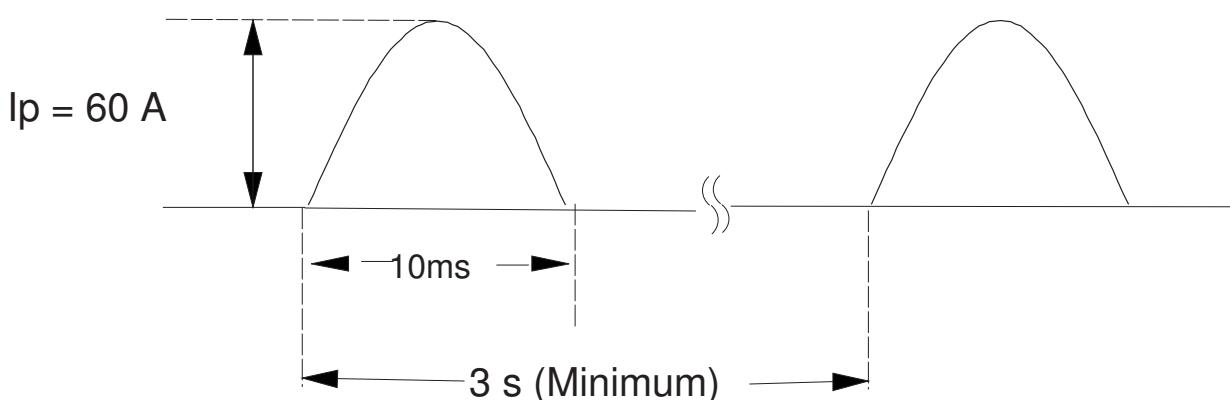
Fig.1. Repetitive surge conditions.  $I_p=60\text{A}$  ( $f=50\text{Hz}$ ) at  $T_c=45^\circ\text{C}$ . Maximum number of cycles  $n=100\text{k}$ . Repetitive cycle  $T=3$  seconds minimum.
