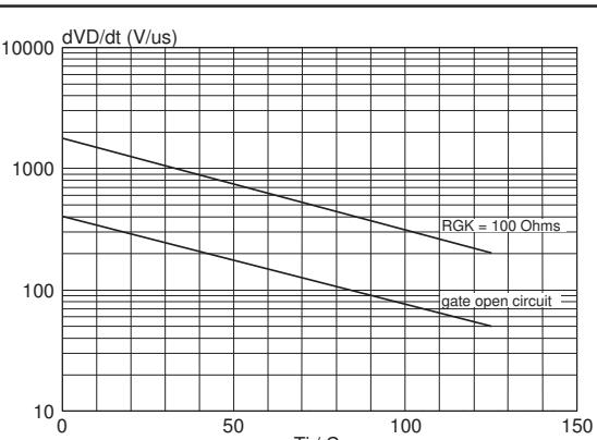
Fig.13. Typical, critical rate of rise of off-state voltage,
