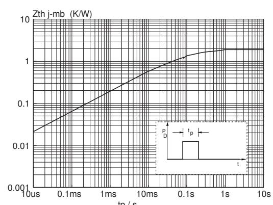
Fig.12. Transient thermal impedance  $Z_{th\ i\cdot mb}$ , versus pulse width  $t_p$ .
