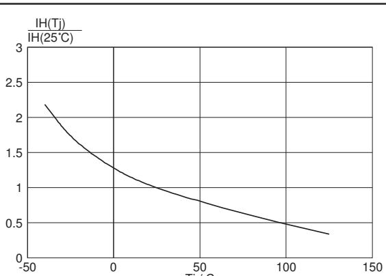
Fig.10. Normalised holding current  $I_H(T_j)/I_H(25^\circ C)$ , versus junction temperature  $T_j$ .
