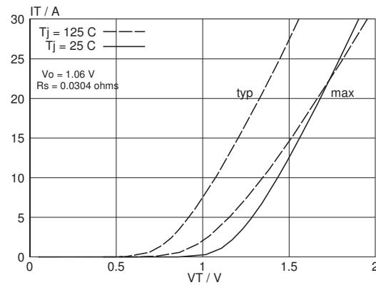
Fig.11. Typical and maximum on-state characteristic.
